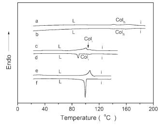
**FIGURE 1** DSC traces (10 °C/min) recorded during the second heating scan (a), the first cooling scan (b) of 1; the second heating scan (c), the first cooling scan (d) of 2; and the second heating scan (e) and the first cooling scan (f) of 3.
