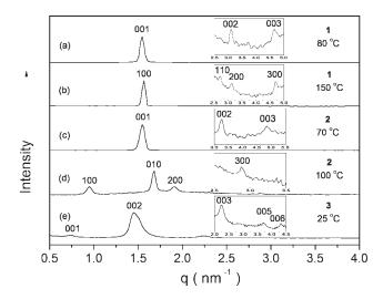
**FIGURE 3** Small-angle X-ray diffraction patterns of **1**, **2**, and **3** measured in solid state and melt state plotted against  $q (= 4\pi \sin \theta/\lambda)$ . (a) in the lamellar phase for **1** at 80 °C, (b) hexagonal columnar phase for **1** at 150 °C, (c) lamellar phase for **2** at 70 °C, (d) rectangular columnar phase for **2** at 100 °C, and (e) lamellar phase for **3** at 25 °C.
