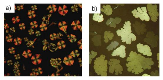
**FIGURE 2** Representative optical polarized micrograph ( $\times$ 100) of the texture exhibited by (a) hexagonal columnar structure of **1** and (b) rectangular columnar structure of **2** at the transition from the isotropic liquid. [Color figure can be viewed in the online issue, which is available at www.interscience.wiley.com.]
