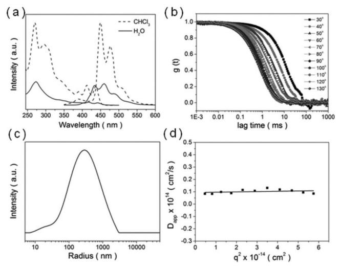
**FIGURE 5** (a) Absorption and emission spectra of **3** in  $CHCl_3$  and aqueous solution (0.002 wt %), (b) autocorrelation functions of **3** in aqueous solution (0.01 wt %), (c) hydrodynamic radius distribution of **3**, and (d) angular dependence of diffusion coefficient for **3**.
