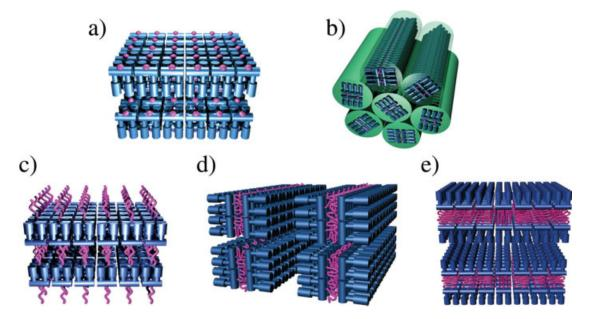
FIGURE 4 Schematic representation of self-assembly of (a) monolayer structure for 1, (b) hexagonal columnar structure for 1, (c) monolayer structure for 2, (d) rectangular columnar structure for 2, and (e) bilayer structure for 3.
